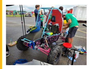
Our goal is to deliver **reliability** and **maneuverability** in harsh environments with a rugged suspension package, a custom-designed gearbox and differentials, and a rear-wheel cutting brake, and emphasize **innovative performance** with, among other features, a custom electromechanically-actuated continuously-variable transmission system.
